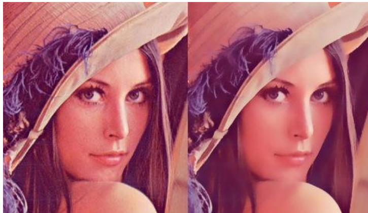
Figure 5 - A bilateral filter applied to a 2D image. The left picture is the original image. The right picture has the filter applied to it, resulting in noise removal.
