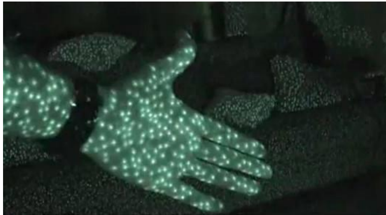
Figure 4 - The infrared pattern emitted by Kinect
